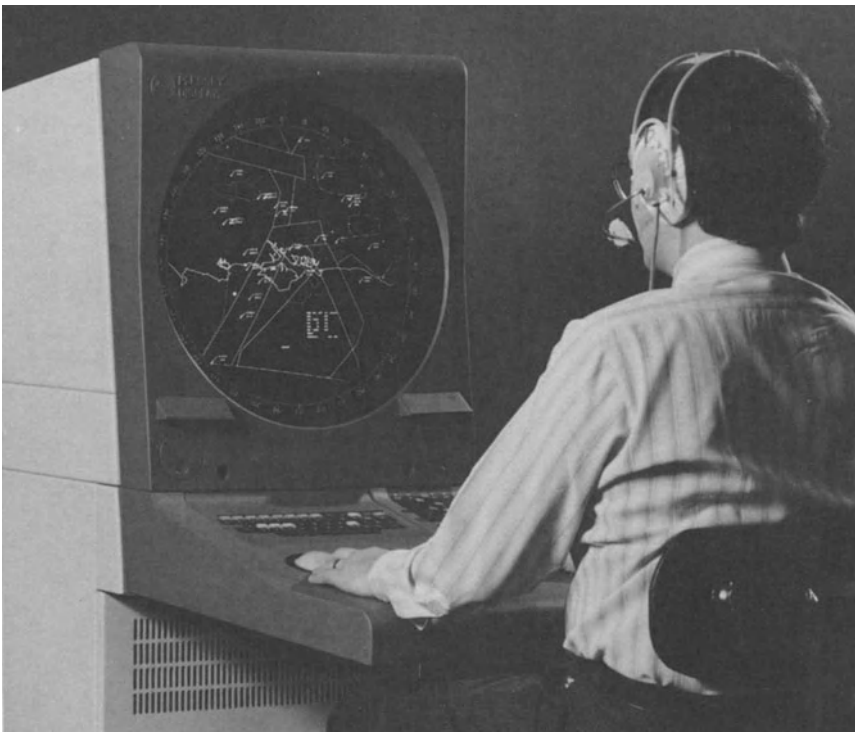
Figure 5.18 A modern synthetic PPI display. Note the hand-operated tracker ball used by the operator to control symbols on the display (photo courtesy of Plessey Radar Ltd)
