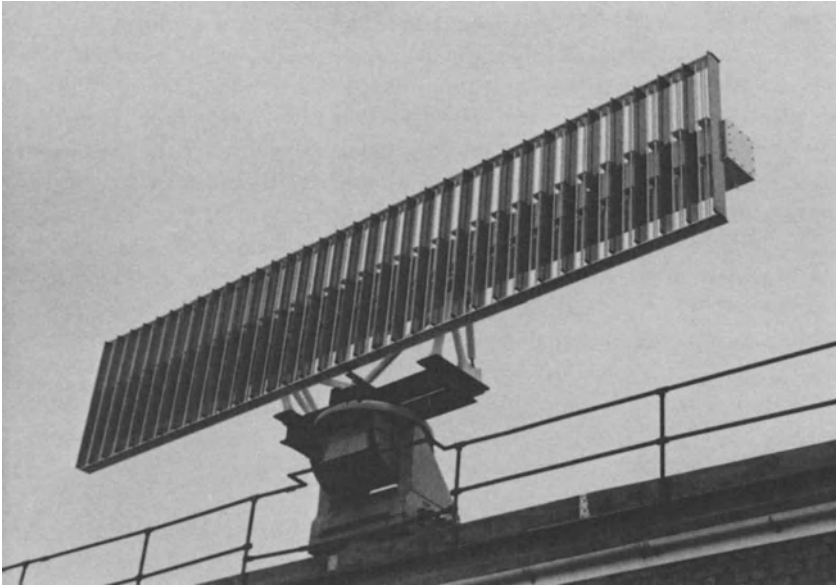
Figure 6.4 A large-vertical-aperture (LVA) antenna for secondary surveillance radar (photo courtesy of Cossor Electronics Ltd)
